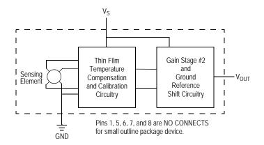
Figure 1. Fully Integrated Pressure Sensor Schematic
