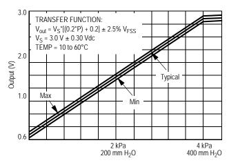
Figure 4. Output versus Pressure Differential at ±2.5% V<sub>FSS</sub> (See Note 5 in Operating Characteristics)
